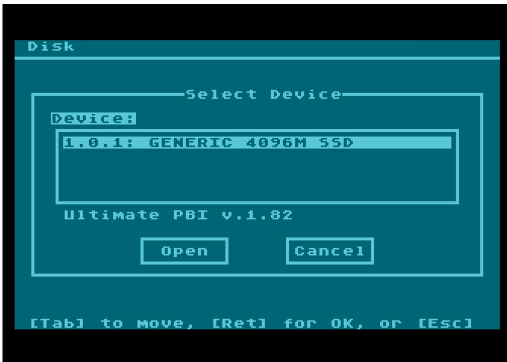
The device selector lists every single APT block device on the system, whether a PBI controller or LSIO-attached device driver. It’s therefore possible to run different physical devices via different adapters at the same time. Most commonly, though, you will see only one entry here: PBI, controller
