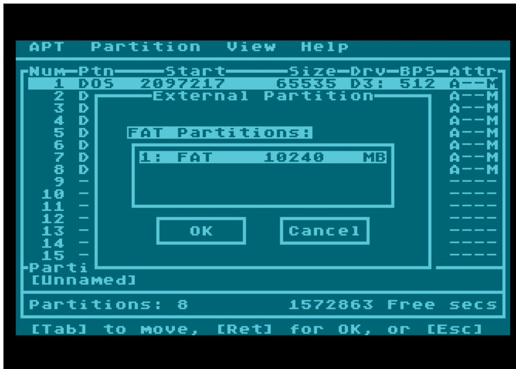
We can see the FAT16 partition we created earlier (although it's currently unformatted – we'll do that on the PC later), so hit return and an entry pointing to that FAT will be added to the APT table. The external partition is denoted by a left-pointing wedge at the left side of the entry. All that remains is to assign the external partition a drive number.
